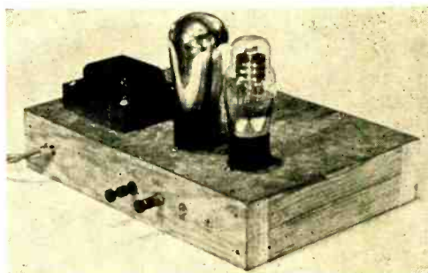
Figure 13. An experimental model of a pulse generator using the circuit of figure 12.
