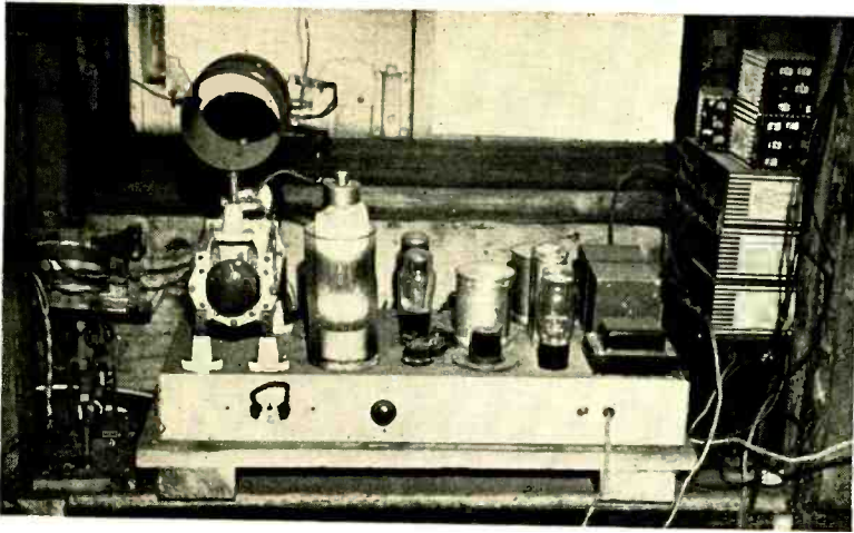
Experimental ionosphere measurement transmitter as installed at West Virginia University.
